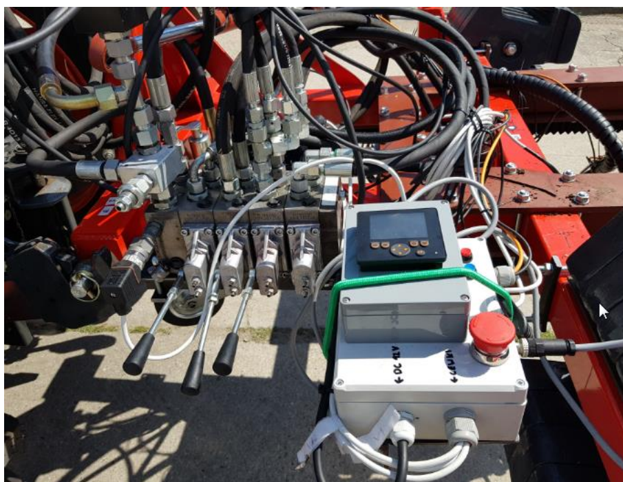
Figure 4 Controller, display and valve block
