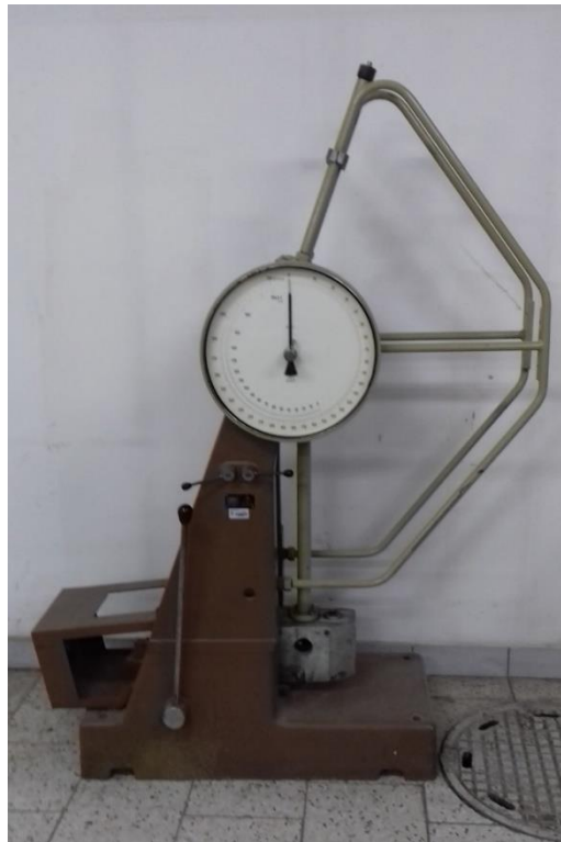
Figure 6 Impact testing machine used in this study
